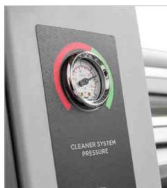
Display for rollers pressure of the cleaning system
