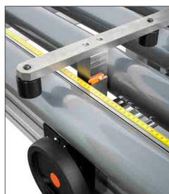
Side adjustable reference bar for the right positioning of the substrate to laminate
