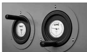
Manual lifting of the top laminating cleaning roller and the lamination roller (motorized optional)
