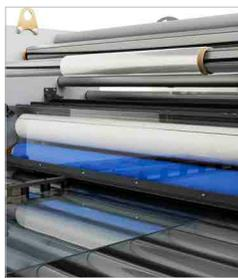
Contact cleaning system of the substrate to laminate with antistatic bar to remove dust from the surface
