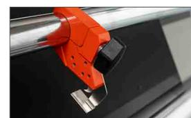
Cutting unit to trim the film if wider than the plate
