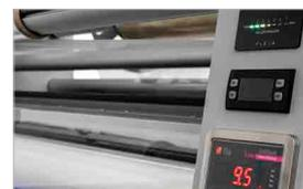
Load tensioning control of the film: it keeps the same tension regardless of roll diameter (optional)
