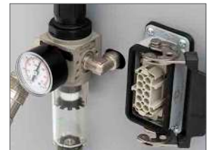
Connectors to eventually connect an external cutter for sheeting
