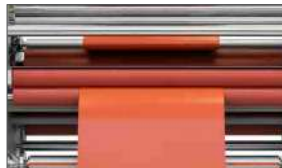
Rear traction rollers with pneumatic lifting and manual control
