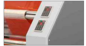
Accurate tensioning adjustment of the steel plate and silicone roll with loading cell
