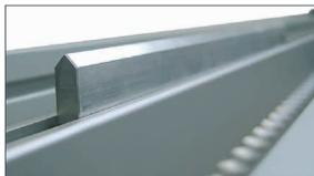
Accessory for bending sheets of 0,5 mm thickness (optional)
